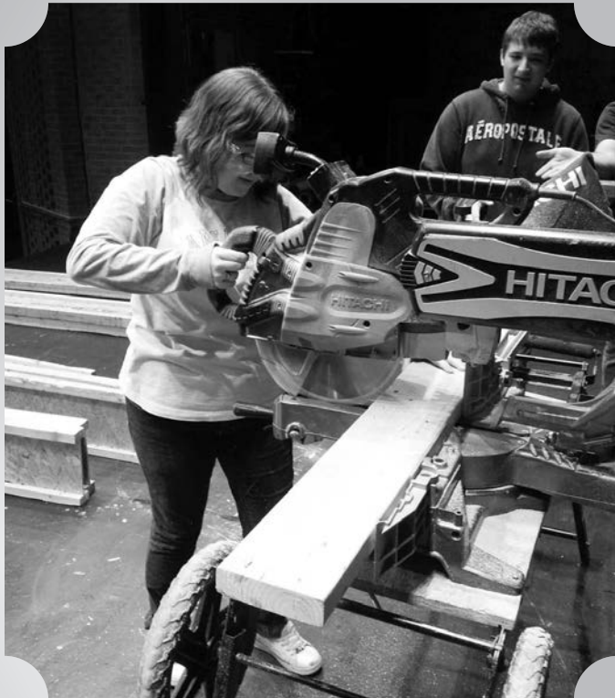
Theatre major Veronica Justice uses a heavy duty miter saw to cut a board for the spring musical set during a recent Technical Theatre class at RLC.
