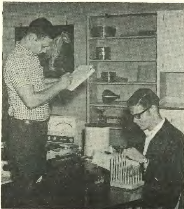
SOIL TESTING is a major concern of the students in Agricultural Business. Here Bill Scott uses a pH meter while Marshall Mills operates the flame photometer. In the foreground is the colorimeter, which is often used in conjunction with the flame photometer.
