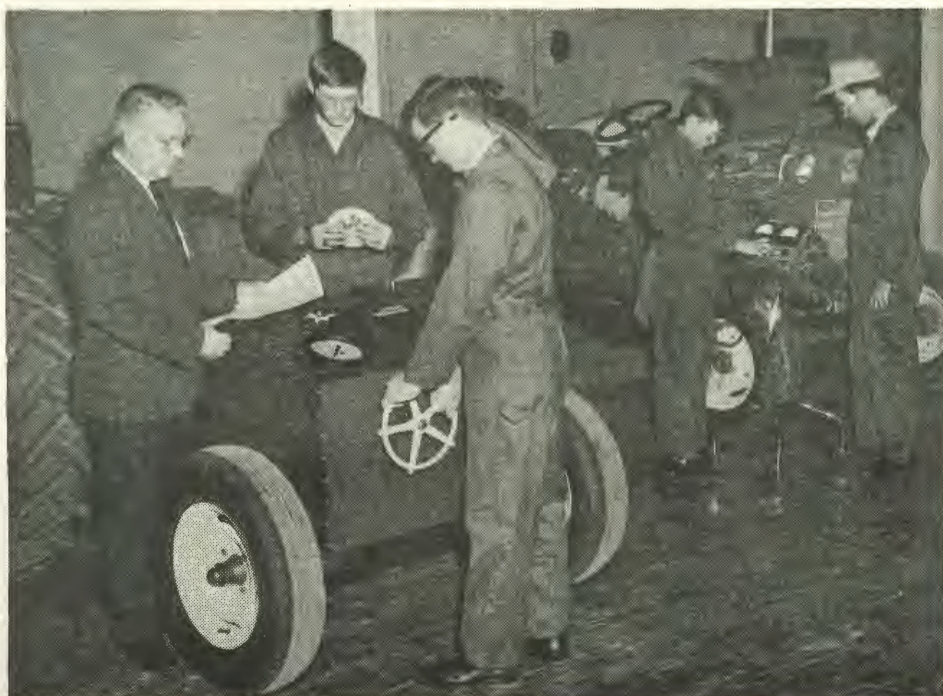
TESTING THE HORSEPOWER of a tractor requires a bit of manpower. As Agricultural Coordinator Ardell Kimmel gives instructions, David Meyers prepares to read the results. Gary Simmons is turning down the valve on the dynameter. In the background are Larry Bealty and Charles Allen as they check the engine of one of the other tractors.
